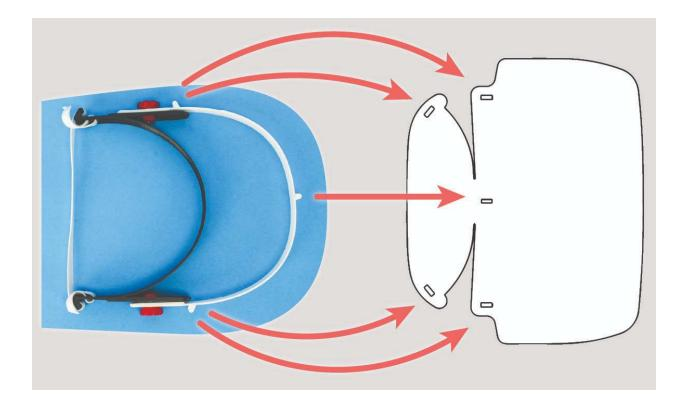
Start with the slot on one side and follow with the slot in the middle. These two should be easy.
